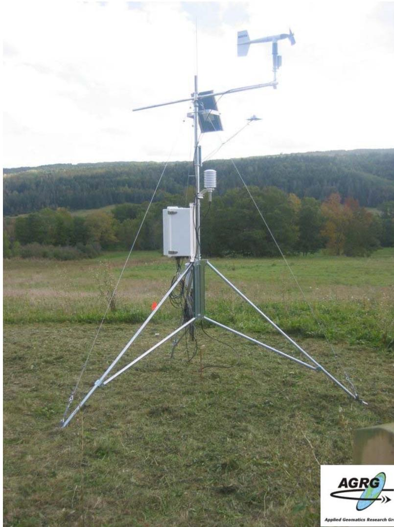
Figure 2 – AGRG weather station tripod setup in the Grand Pre area (photo facing south east).
